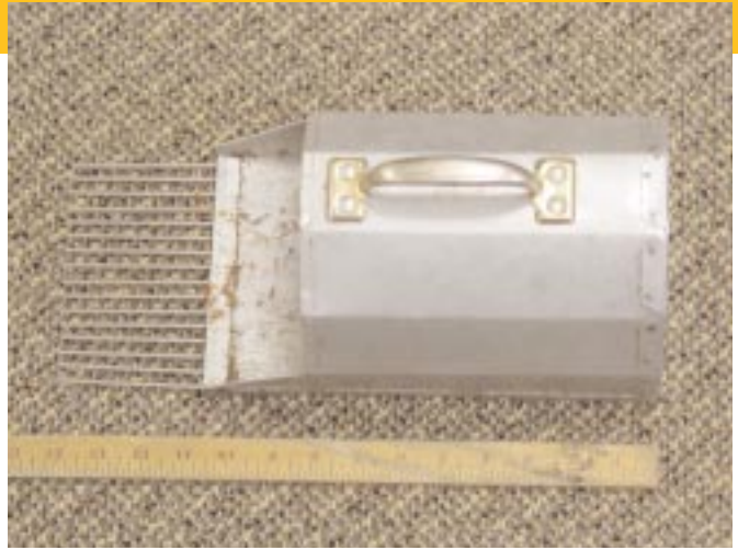
Figure 2. A custom-made metal harvester for collecting fruits.
