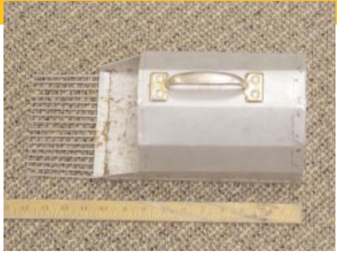
Figure 2. A custom-made metal harvester for collecting fruits.
