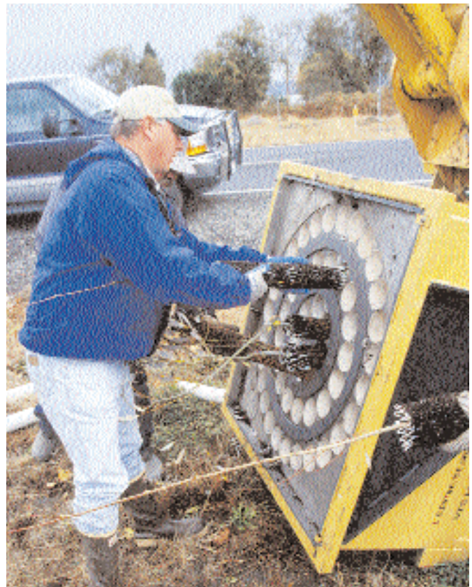
Figure 5. The expandable stinger working on a riparian project and loading the “50-shot” head, Central Point, Oregon.
