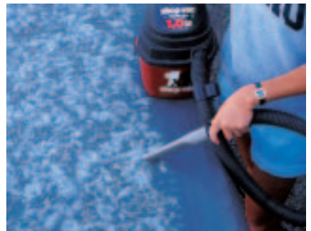
A 1-horsepower shop vacuum sucks the cotton and seeds through the window screen—coarser debris remains behind. Inside the vacuum, the cotton sticks to the cloth filter and the seeds collect in the bottom of the canister.
