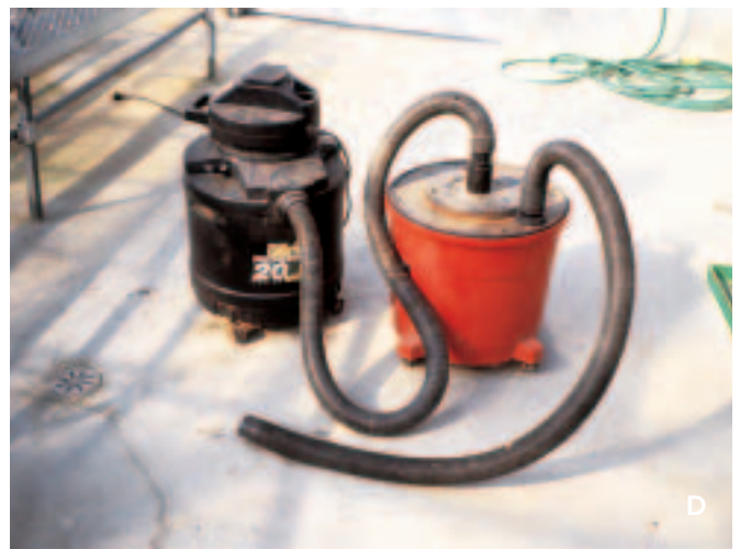
Figure 2. Wooden racks with either flyscreen (on the bottom) or 1 cm (0.375 in) hardware cloth (on the top) hold aspen capsules as they release cotton and seeds (A). Cotton and seeds are vacuumed from the wooden racks (B) using a 5-horsepower shop vacuum. The vacuum pulls the seeds into a passive shop vacuum canister that has been modified 2 ways: the motor has been removed and replaced with a connector pipe and the exit pipe has 2 openings (C). The seeds drop out in the passive canister and the cotton is vacuumed into the second shop vacuum with the motor (D).
