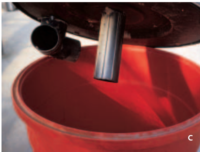
Figure 2. Wooden racks with either flyscreen (on the bottom) or 1 cm (0.375 in) hardware cloth (on the top) hold aspen capsules as they release cotton and seeds (A). Cotton and seeds are vacuumed from the wooden racks (B) using a 5-horsepower shop vacuum. The vacuum pulls the seeds into a passive shop vacuum canister that has been modified 2 ways: the motor has been removed and replaced with a connector pipe and the exit pipe has 2 openings (C). The seeds drop out in the passive canister and the cotton is vacuumed into the second shop vacuum with the motor (D).
