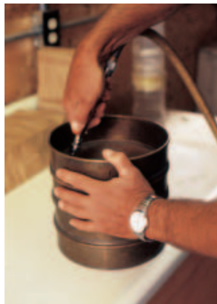
Figure 3. Three soil sieves are needed to clean seeds. The bottom sieve is where the seeds collect. Cotton and seeds are placed in the middle sieve. The top sieve holds the cotton from blowing out when a stream of compressed air is blown across it. The cotton remains in the middle sieve and clean seeds are deposited in the bottom.
