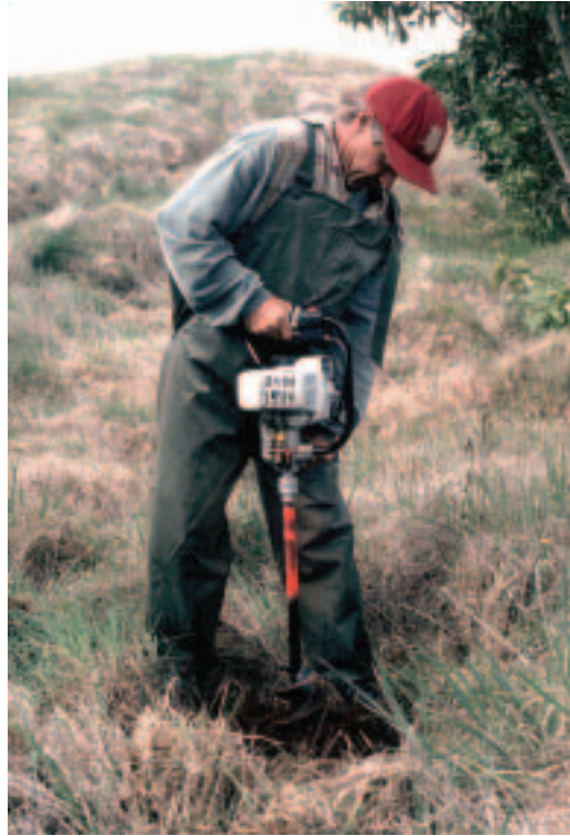
Figure 1. A gasoline-powered engine drill fitted with a large bit facilitates planting stock grown in larger containers.
