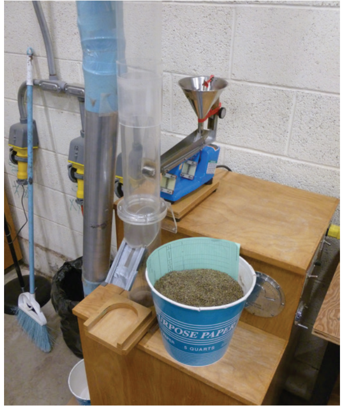
Brushed (Westrup LA-H brush machine) yellow Indian paintbrush seed-bearing material ready to be passed through an air column separator (background) to separate chaff from seed.
