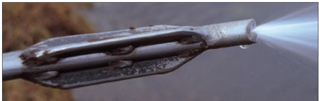
Figure 5 • Vanes on the probe, just above the nozzle, enhance performance in clay and silt soils.
