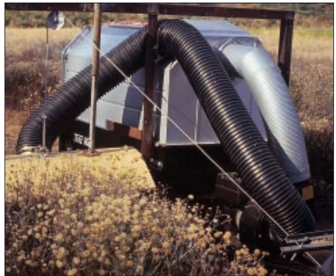
Figure 1 • Left: The pull-behind leaf vacuum and the plywood hood sized to fit over a row of native seeds. Right: Harvesting fluffy seeds.
