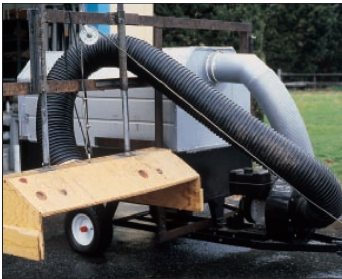
Figure 1 • Left: The pull-behind leaf vacuum and the plywood hood sized to fit over a row of native seeds. Right: Harvesting fluffy seeds.
