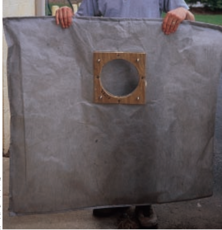
Figure 2 • Tyvar seed bag modified with plywood supports that connect to the hose discharge inside the leaf vacuum.
