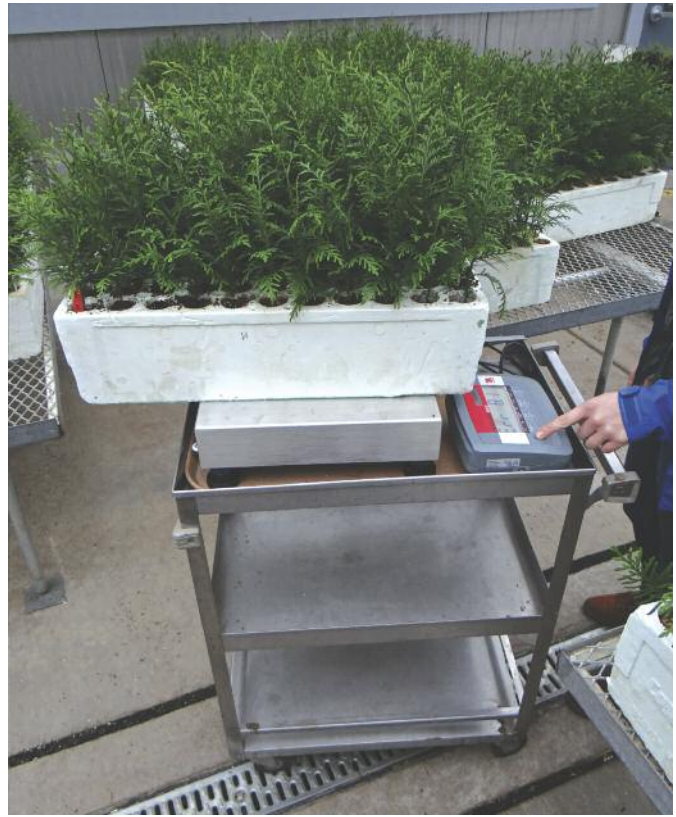
Figure 2. A balance on a cart can be rolled to various locations within the nursery, reducing the amount of time spent transferring containers to and from the balance. Photo by R Kasten Dumroese
