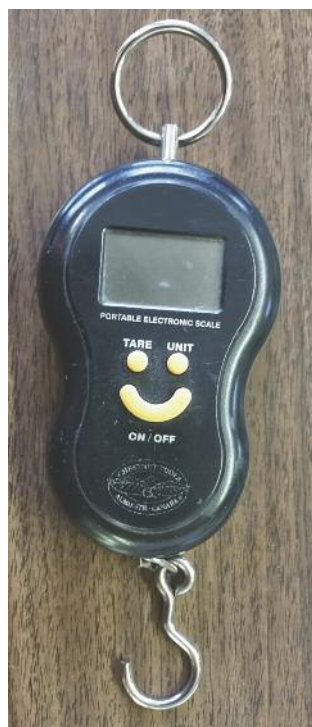
Figure 3. A balance left in place to measure container weights requires no movement of containers or balances, but many balances are needed when multiple species and stocktypes are produced. Photo by R Kasten Dumroese
