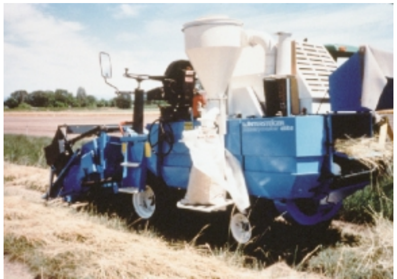
Figure 3 • A Nursery Master Elite 140 plot research combine (Wintersteiger, Salt Lake City, UT) combining swathed Elymus glaucus .
