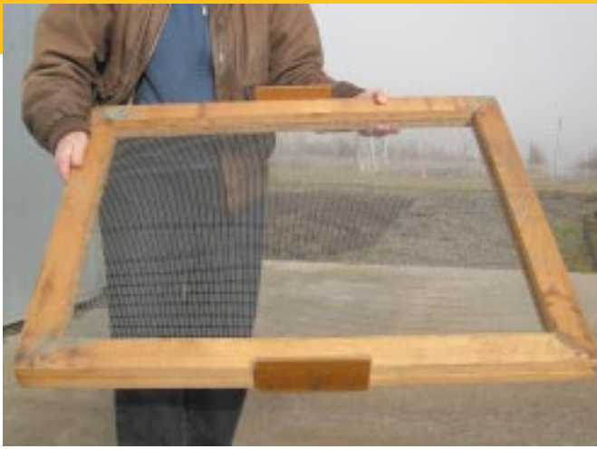
Figure 2. A wooden frame covered with hardware cloth makes an effective grass seed cleaning device.
