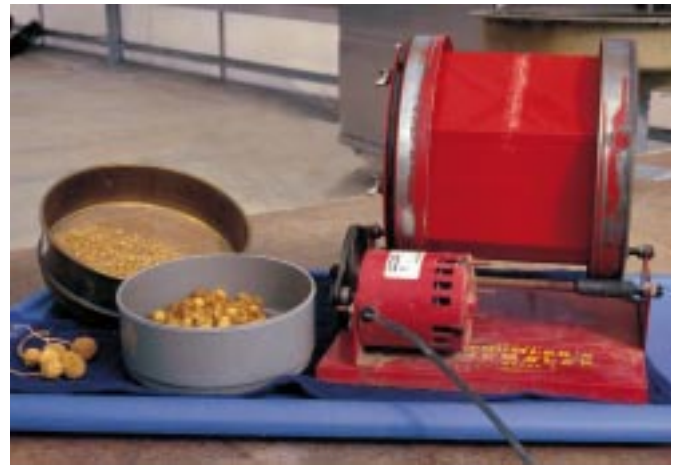
Figure 2. At Los Lunas Plant Materials Center, dry fruiting heads of Arizona sycamore, seen lower left, are crushed under water in a large pan. The hairs agglomerate into balls (gray sieve in foreground). A slurry of achenes and pea gravel are tumbled in the rock tumbler to dislodge the hairs. Finally, the achenes, hairs, and pea gravel are separated with soil sieves with the cleaned achenes visible in the brass sieve (background).
